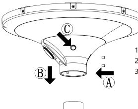
1. Insert the lamp into the lamp pole (Figure B)
